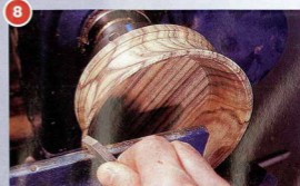
8 You can form quite a crisp bead on the rim of the coaster by simply dabbing at the corners with the beading tool
