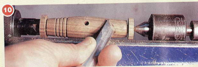
You get a very clean finish with a skew chisel, as long as you are cutting with the grain
