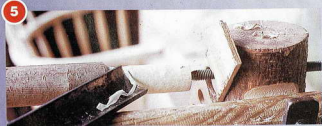
The one-inch pegs on the legs can be cut with a rounder or turned on a lathe - in this case, a proper rustic pole lathe
