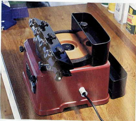
The grinder with its blade sharpening jig attached and ready for action
