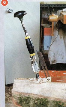
When you're drilling the leg sockets into the seat, a bevel will prove a useful aid to guiding the angle
