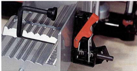
The ratchet-style work clamp on the Nobex is well made, but cannot be used satisfactorily for overhead clamping
