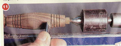
The V is enlarged, and some minimal decoration created, with the point of the skew chisel
