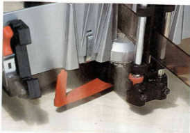
The Nobex saw has a brilliant stepless pivot arm lock lever – which is needed to true up the blade to the 90-degree preset
