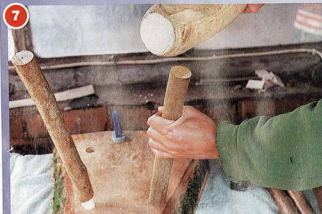
The legs are glued and driven home with a mallet, then wedged from the top
