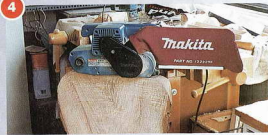
Once you've worked the seat, a belt sander will quickly tidy up the end grain and other rough areas
