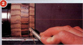
2 Carefully slice the edge of the disc true, using the small bowl gouge
