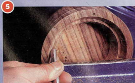
5 Slice down the inside of the opening with the gouge, forming the splayed sides of the coaster
