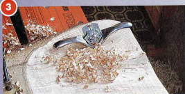
...before finishing off with a convex spokeshave, which allows more precision and will leave some nice rustic tool marks
