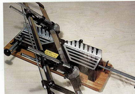
ABOVE & BELOW: CK's 1129/2 in compound mitering mode. The pivot arm lock lever is neat; note the hacksaw-type blade retention
