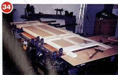
The side frame-and-panel assemblies are glued together in two halves
