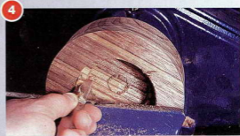
4 Feed the square scraper down the side of the opening, taking small, manageable cuts
