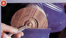
3 You can disguise the dovetail by forming low relief mouldings in and around the recess
