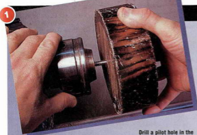
1 Drill a pilot hole in the blank then screw it on to the screw chuck
