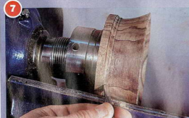
7 Use the point of the spindle gouge to form the tiny corvette moulding in the plinth
