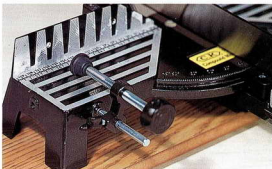
ABOVE & BELOW: The work clamps on the Axminster, CK and Draper saws vary in quality, but can all be used with ease for overhead clamping
