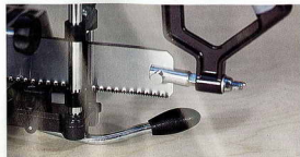
Draper's pivot arm lock lever looks good, but falls short of the standard set by the others
