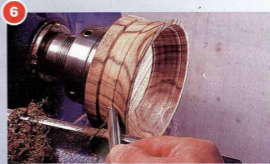
6 Create the moulding on the outside and plinth by taking a number of small cuts
